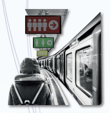
Poles with information near the bus stop indicate the crowding rate to the passengers waiting to board. Equipped with colored LED for the state system, the poles indicate to the passengers which carriages to choose, before the train arrives.
